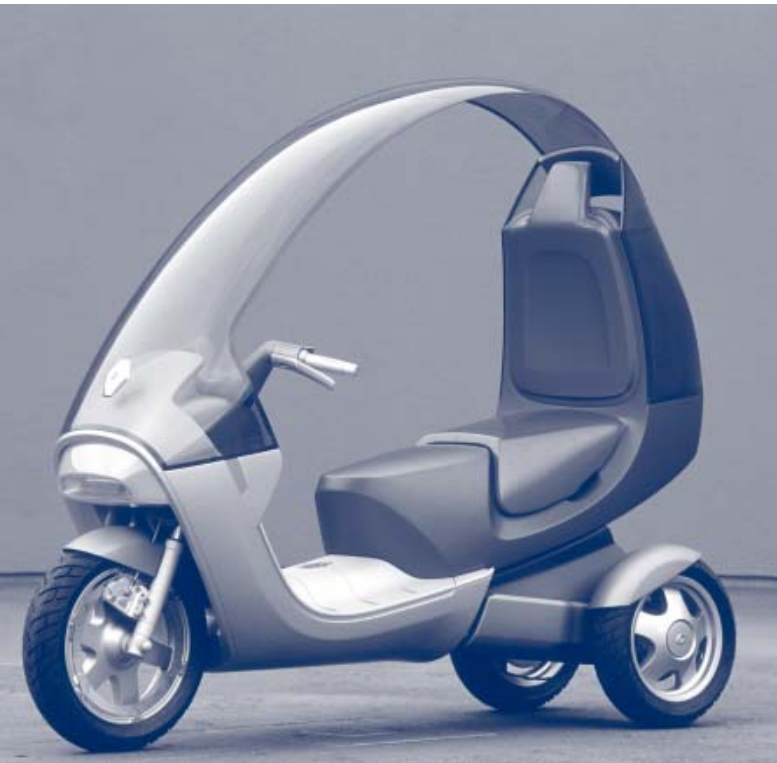
Ublo is a three-wheel concept vehicle mid-way between a two-wheeler and a car. The vehicle can be equipped with a hybrid drive.
